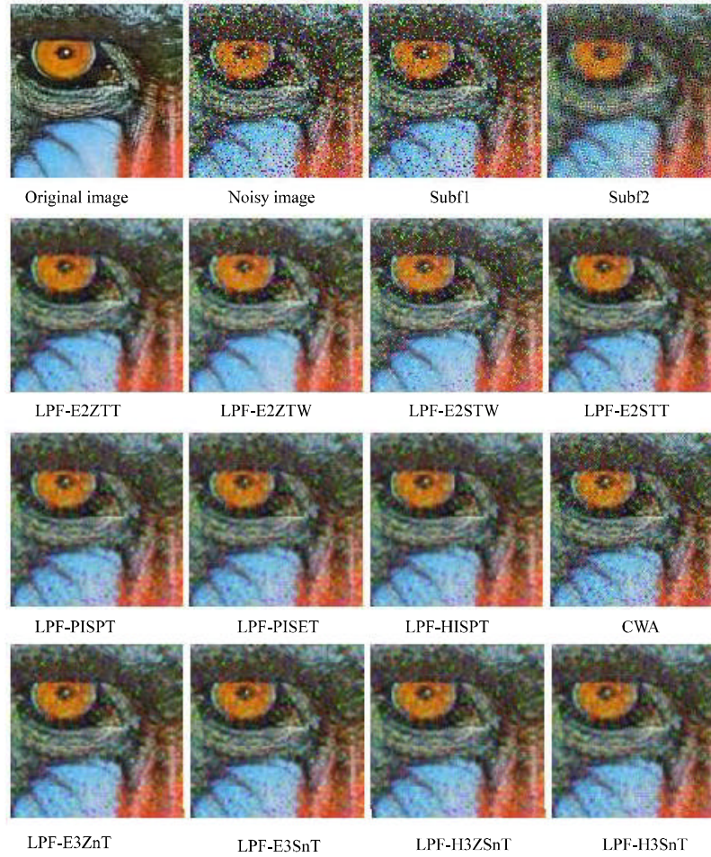
Fig. 9: Part of baboon image with 15% impulse noise (salt and pepper) and the filters output
