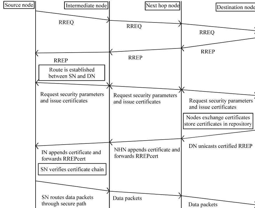
Fig. 1: Design of black hole and worm hole secure framework in MANET
