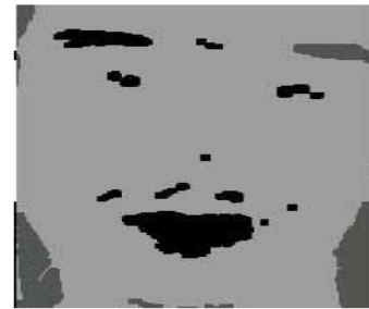
Fig. 4: Erosion applied over dilate representation of the skin-tone representation
