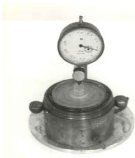
Fig. 2: Test of inflation in a free cell oedometer (without piston)
