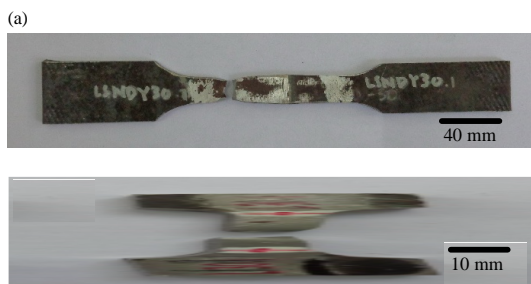
Fig. 12: Fracture of tensile tests; a) Transverse direction and b) Longitudinal direction
