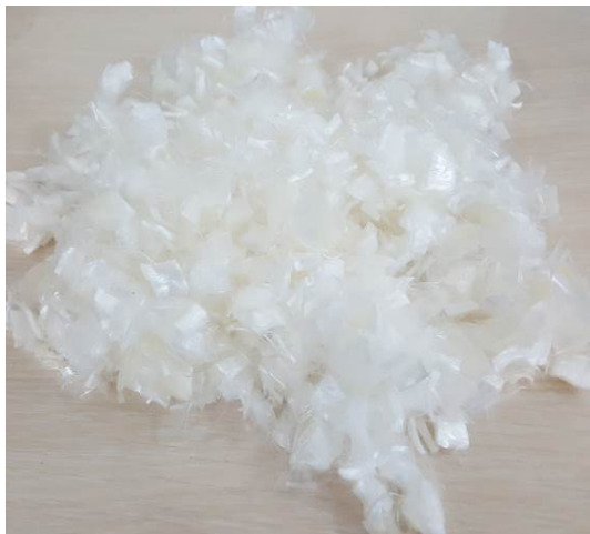
Fig. 2: PP cotton fiber materials
