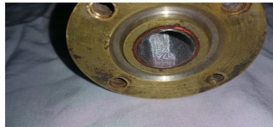
Fig. 2: Wick turn inside heat pipe
