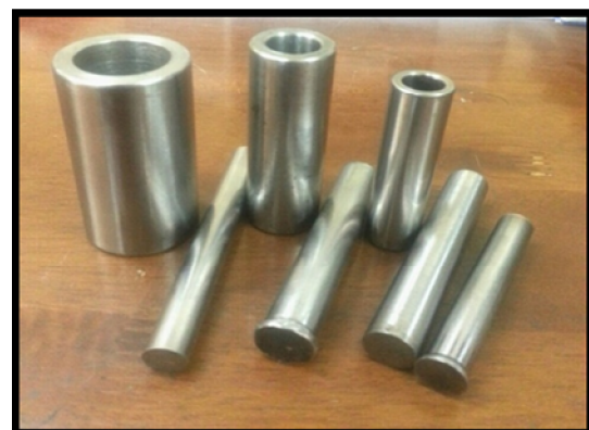
Fig. 5: Die, punch and holder for mold
