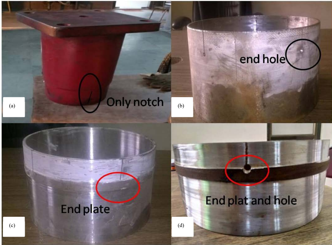
Fig. 2(a-c): Buffer casing prototype with (a) only notch (S1), (b) a hole drilled at the end of notch (S2), (c) with enhancement of 1 mm wall thickness at the notch end (S3) and (d) with enhancement of 1 mm wall thickness and a hole at the notch end (S4)
