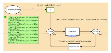
Fig. 2: Hierarchical model of POP synthesis
