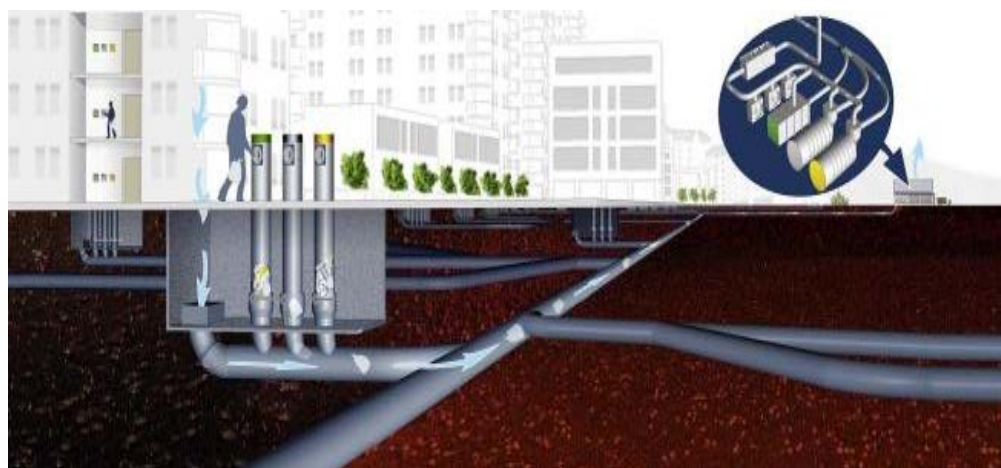
Fig. 13: The scheme of vacuum waste disposal, characteristic for Sweden and Finland
