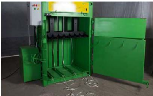
Fig. 12: Waste plastic/aluminum cans bailing machine
